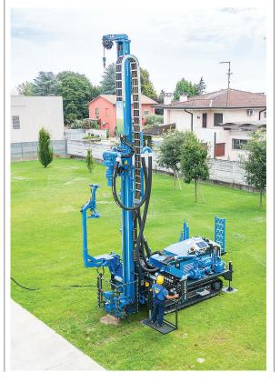
Fraste's FS 500 drilling rig features advanced radio remote controls, streamlining operations from a safe distance and boosting productivity.
